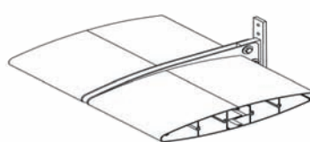
Console fixing brackets are available for 0°, 15°, 30° and 45° blade inclinations. Customised angles available upon request.
