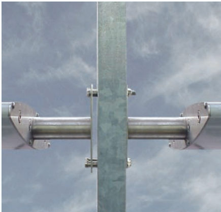
▲ Parallel offset fixing bracket. Shown is a detailed view of an 90° parallel off-set fixing bracket attaching a c|sairfoil AF 270F blade onto a vertical support segment. The brackets are screwed directly onto the end of the blade thanks to the special screw channels incorporated into the extrusion. The bracket-blade unit is then fixed with bolts onto the support segment. The availability of parallel off-set fixing brackets and compound angle fixing brackets in a wide variety of angles cater for an unlimited range of design possibilities and adapt to virtually any project specifications.
